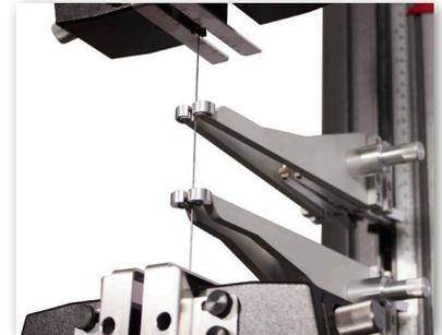
Carbon Fiber Tow in Pneumatic Side-Action Grips with AutoX750
