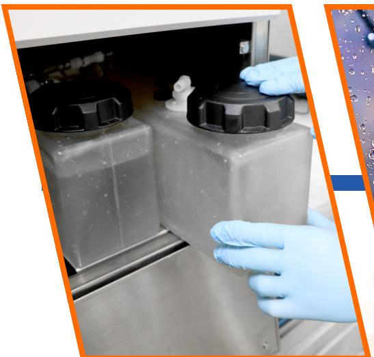
Dual tanks hold 2 acid free TerraBlends that are recirculated, processing hundreds of samples per tank\*. TerraBlend life indicator is customizable to alert users simplifying routine maintenance.
