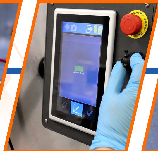
Select your etch area using the joystick and laser indicator. The etch area rectangle can be large or small and placed anywhere on the sample.
